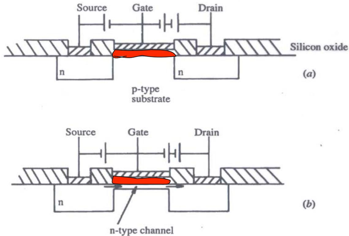
Fig. 7.15 Structure of metal oxide semiconductor field effect transistor (MOS-FET). (a) Gate forward biased with respect to its source. Drain forward biased with respect to gate. (b) Gate reverse biased with respect to its source.
