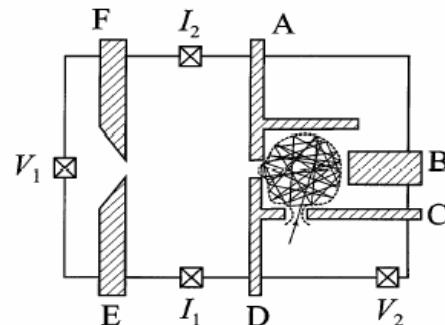
FIG. 1. Schematic top view of the sample structure. The hatched areas show the structure of the Schottky gates, the crosses denote Ohmic contacts. The heating current is passed between  $I_1$  and  $I_2$ . The thermovoltage  $V_{\text{th}}$  is measured between  $V_1$  and  $V_2$ . The chaotic electron trajectories are indicated in the gate-defined dot region (dashed line). An arrow points at the varied quantum-dot lead.
