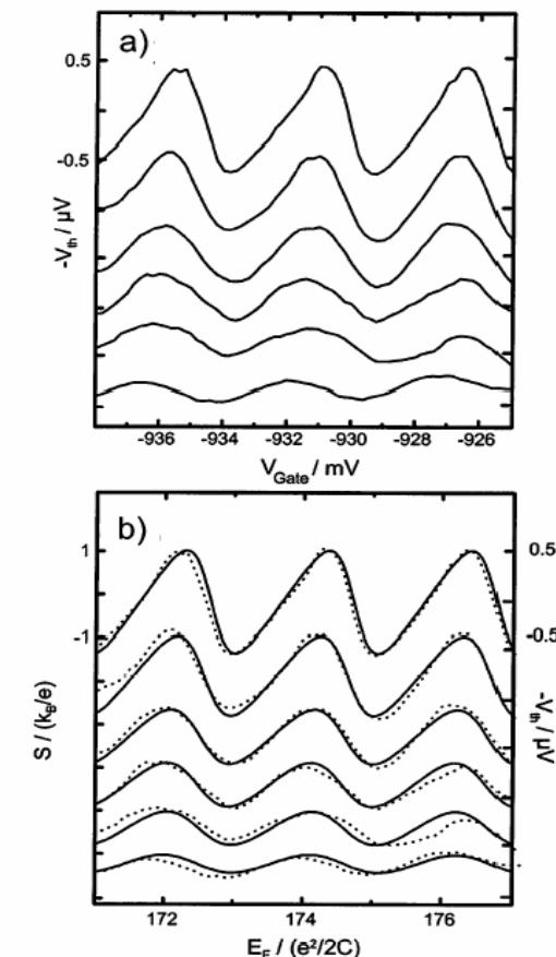
FIG. 2. (a) Experimental traces of the thermovoltage of the quantum dot for a heating current of 40 nA. The transmission probability of point contact  $CD$  was 0.06, 0.19, 0.29, 0.38, 0.43, and 0.82 from top to bottom. (b) Calculated curves of the thermopower of a quantum dot. The values of  $k_B T/E_c$  are 0.22, 0.25, 0.30, 0.33, 0.37, and 0.45 from top to bottom (solid line). The experimental thermovoltage measurements from (a) are added as dashed lines.
