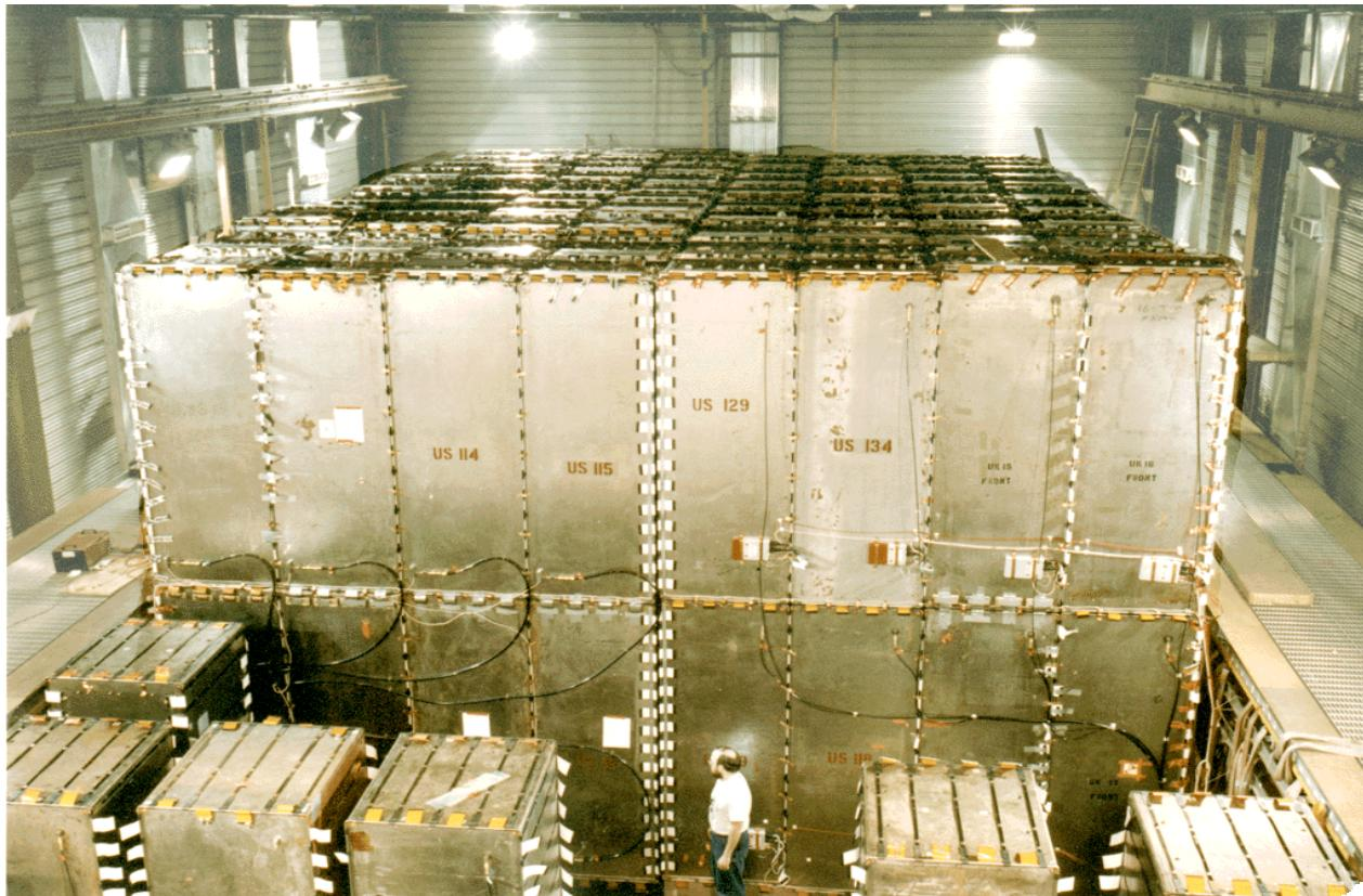
The detector is surrounded by a  $\sim 1700 \text{ m}^2$  “veto shield” which provides nearly  $4\pi$  coverage for the identification of charged particles entering / exiting the detector cavern.
