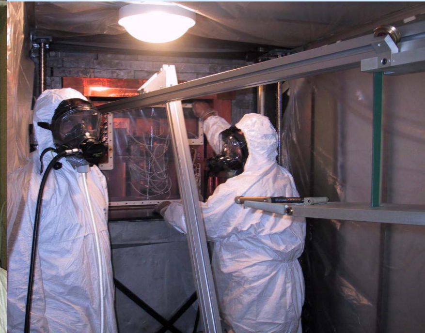
Dismounting the ~100kg NaI(Tl) set-up in August 2002 in HP N 2 atmosphere
