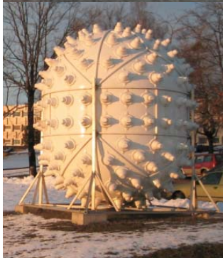
Target: 5 ton liquid scintillator with 0.09% Gadolinium
