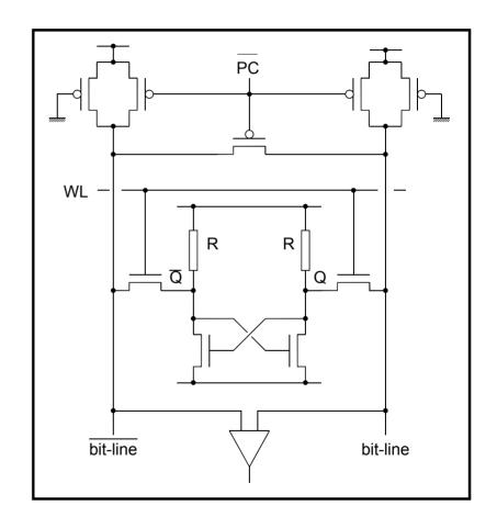
A cross-coupled inverter pair can be used as a sense amplifier
