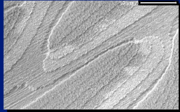
Section of the fabricated 8-level structure of a beamsplitter
