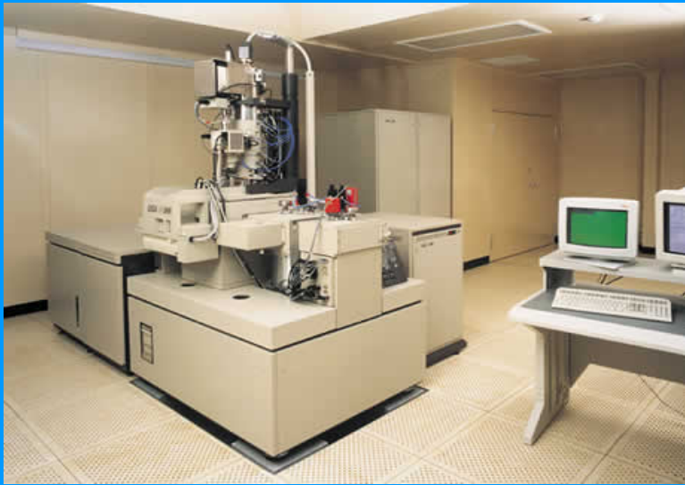
Typical e-beam system used in the production (Leica VB6 HR type)
