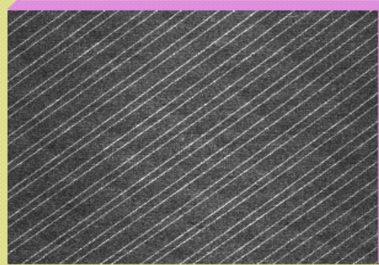
TEM Image: SiO 2 lines (10 nm width) on Si Surface, written by a CNT tip
