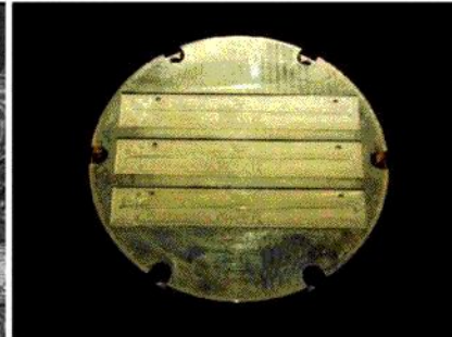
Metal mold insert made of brass
