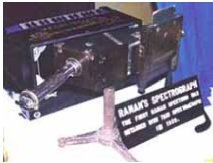
Above: Raman's spectrograph with photographic plate Right: First spectra published in Indian Journal of Physics
