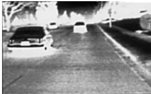
IR image with 240x336 microbolometer camera
