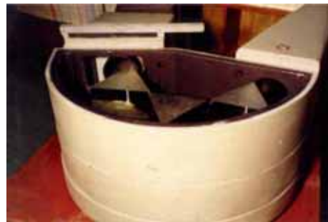
Huet prism (35 cm) spectrograph -1940's
