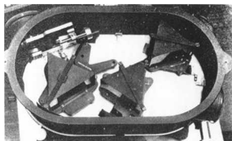
3-4 cm prisms in Steinheil Raman Spectrometer-1957
