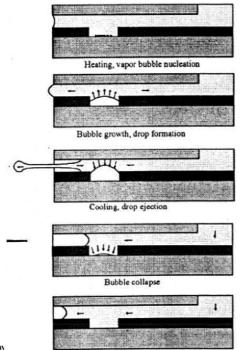
M.P. O'Horo, N.V. Deshpande and D.J. Drake, Drop generation process in TIJ printheads, Proc. 10th Int. Congress on Advances in non-impact printing technologies, Soc. Imaging, Sc. and Techn. (IS&T) 1994, p. 418
