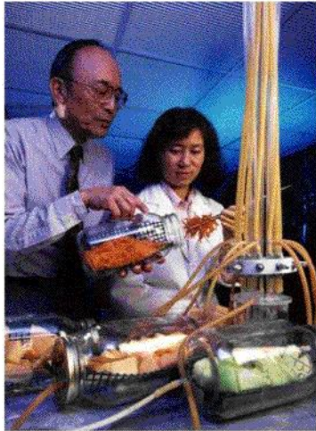
Food technologist prepare e.g. shredded carrots for automated measurement of respiration rate and ethylene production. www.ars.usda.gov
