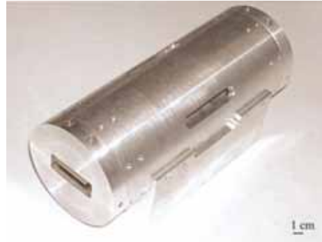
0.6 Tesla mini-magnet; Moresi e.a. Conc. Magn. Res. B Magn.Res. Eng. 19, 35-43 (2003)
