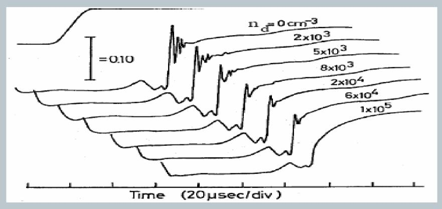
• The oscillatory shock waves were excited in a plasma first without dust and then with dust: as  $n_d$  is increased, oscillatory wave structures behind the shock decreases and completely disappears at  $n_d$ =10<sup>5</sup> cm<sup>-3</sup>.
