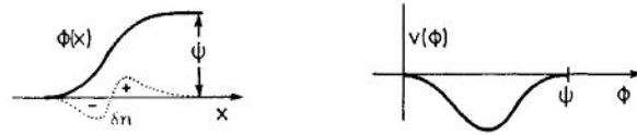
Fig. 14. The electrical and classical potential of a DL. The dotted line represents the dipole-like total charge density.
