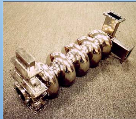
Niobium cavity \sim 0.5 m long (Jefferson Lab).
