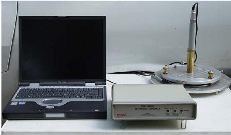
Fig.5. Geomagnetic system configuration
