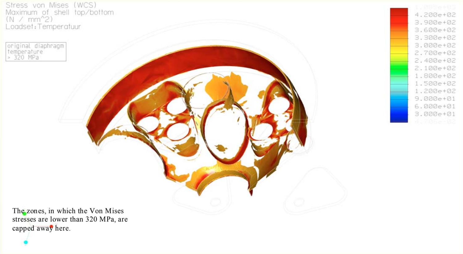
Figure 10. Von Mises stress for thermal load.
