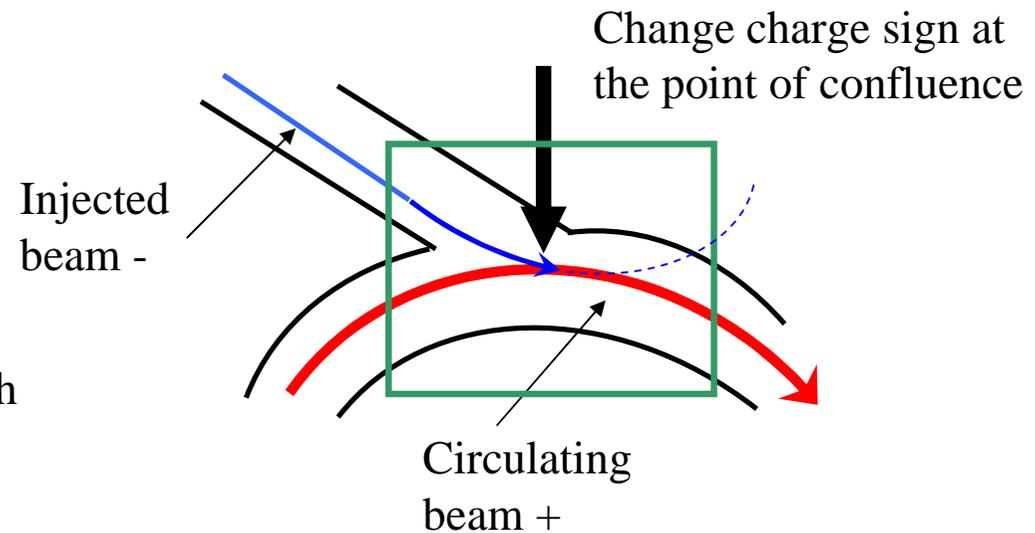
Injection in magnetic field with charge exchange does allow confluence of two beams
