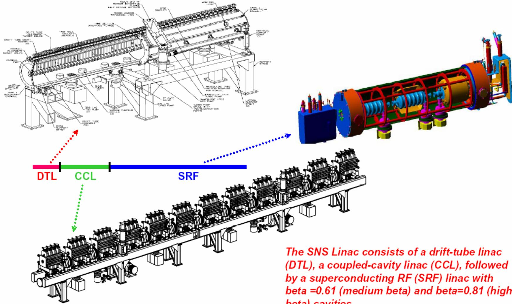
The SNS Linac consists of a drift-tube linac (DTL), a coupled-cavity linac (CCL), followed by a superconducting RF (SRF) linac with  $\beta = 0.61$  (medium beta) and  $\beta = 0.81$  (high beta) cavities.
