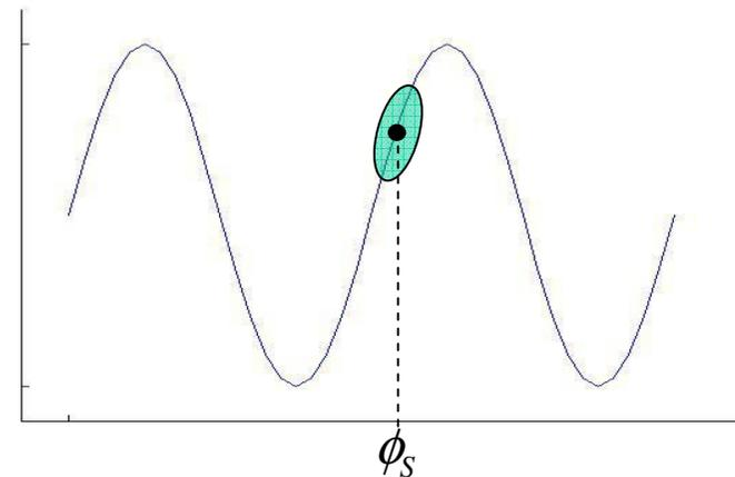
**! Autophasing** mechanism can provide **longitudinal focusing**
