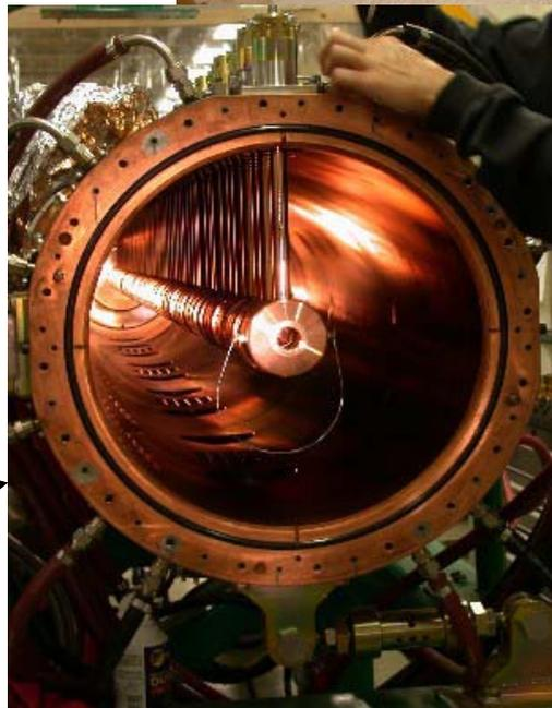
DTL tank with drift tubes installed
