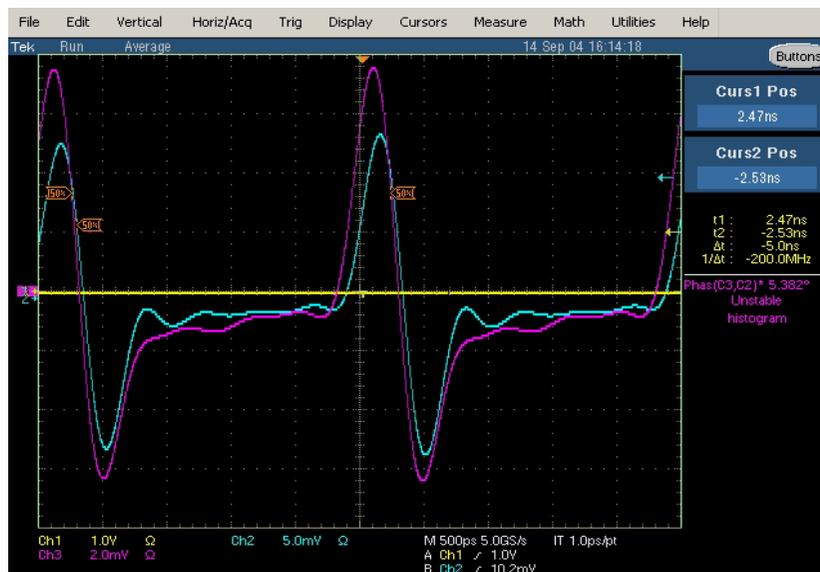
Time of flight energy measurement using a pair of BPMs
