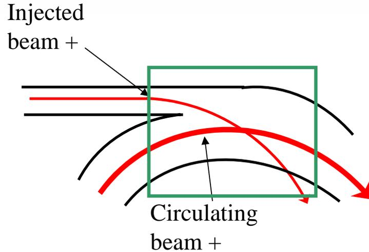
Injection without charge exchange doesn't allow confluence of two beams
