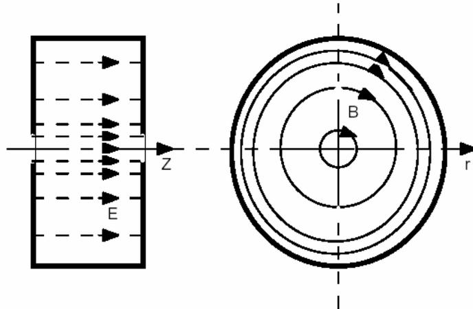
Electric E and magnetic B fields for the lowest mode in a cylindrical (pillbox) cavity resonator.
