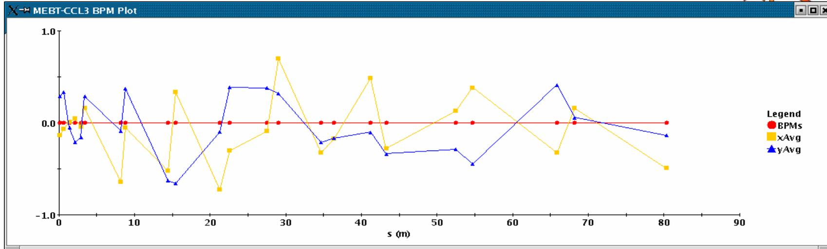
Beam trajectory in the warm linac
