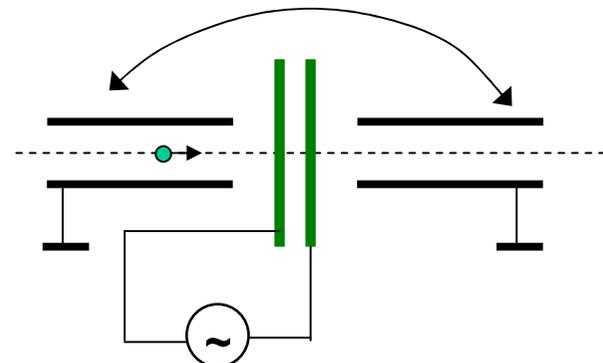
**Radio-Frequency (RF) acceleration principle**
