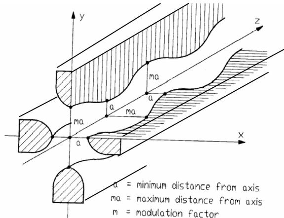
➤ Longitudinal electric field is created by modulating electrode shape along the longitudinal axis
