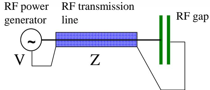
➤ Rf power required to create 100kV voltage in the gap:
