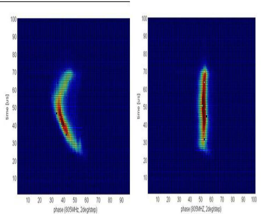
Phase width of the bunch along the pulse with feedback alone (left) and feedback + feedforward (right)
