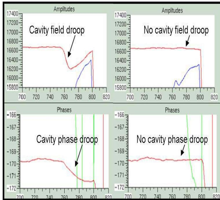
Cavity field and phase droop with feedback alone (left) and feedback + feedforward (right) beam loading compensation.
