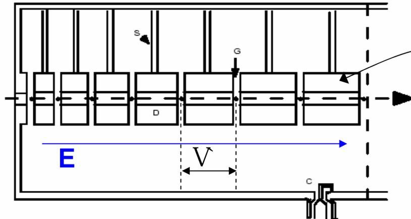
Focusing quadrupoles are inside drift-tubes.
