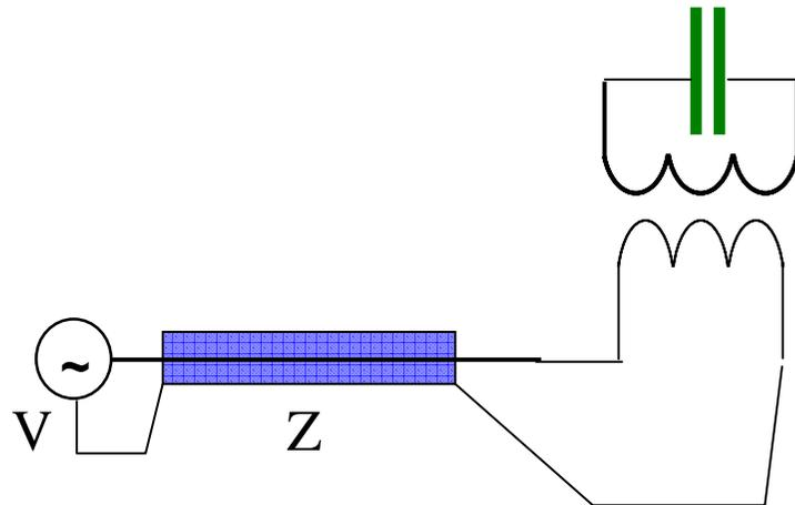
➤ Transformer allows higher voltage without power increase
