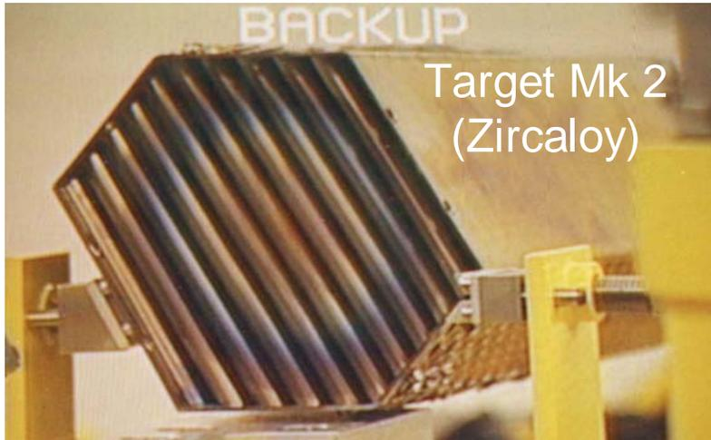
Removed after 6.8 Ah of beam
