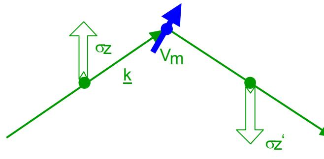
$$\frac{d\sigma}{d\Omega} = (\gamma r_0)^2 \left| -\frac{1}{2\mu_B} \langle \sigma_z' | \underline{\sigma} \cdot \underline{M}_{\perp}(Q) | \sigma_z \rangle \right|^2$$
