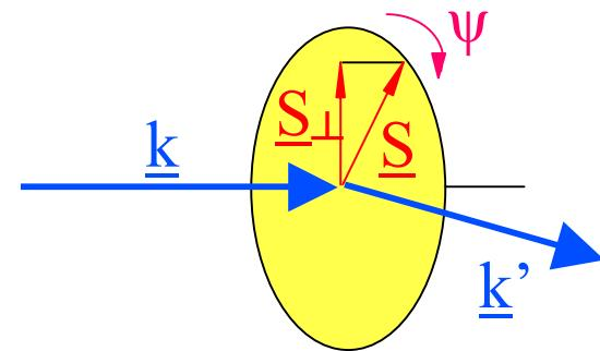
$$\left. \frac{d\sigma}{d\Omega} \right|_{mag} = r_0^2 \left( \frac{\lambda_C}{d} \right)^2 |S_{\perp}|^2$$
