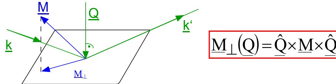
Only the component of the magnetisation perpendicular to the scattering vector gives rise to magnetic scattering!
