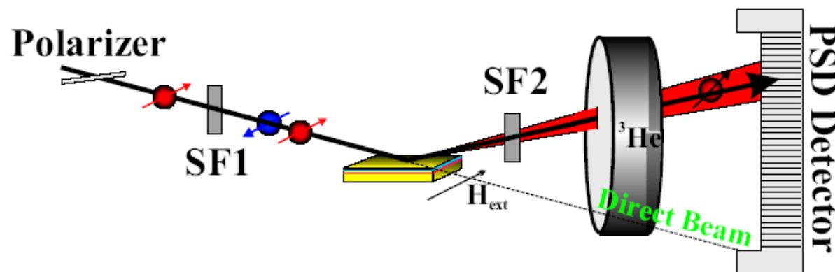
${}^3\text{He}$  spin-filter technique is very useful for the polarization analysis of off-specular scattering. Compared to solid-state analyzer, the spin-filter covers a wider angular range and is free of small angle scattering.
