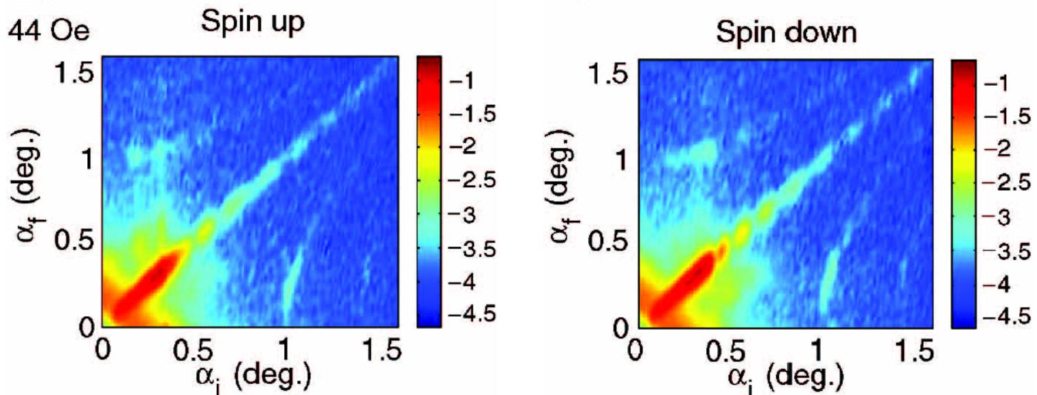
Specular reflectivity ridge can be recognized and off-specular Bragg peaks from the lateral stripe array.
