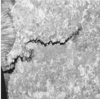
Re-heat cracking in advanced gas cooled reactors
