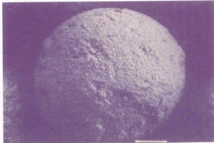
Porous Microsphere (SEM Picture)
