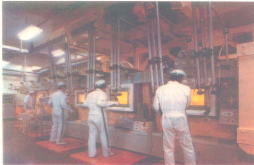
Remote Operations using manipulators for handling highly radioactive materials (mainly high gamma and high neutron dose) inside concrete hot cells
