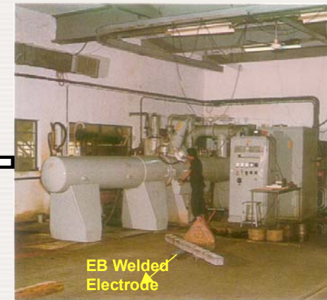
Electron Beam Welding of Briquettes to form Consumable Electrode
