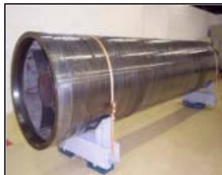
Container for spent fuel
