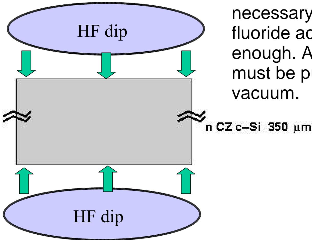
Removal of native oxide is necessary. A simple dip in hydro fluoride acid (HF) is usually enough. After this step the sample must be put immediately into vacuum.
