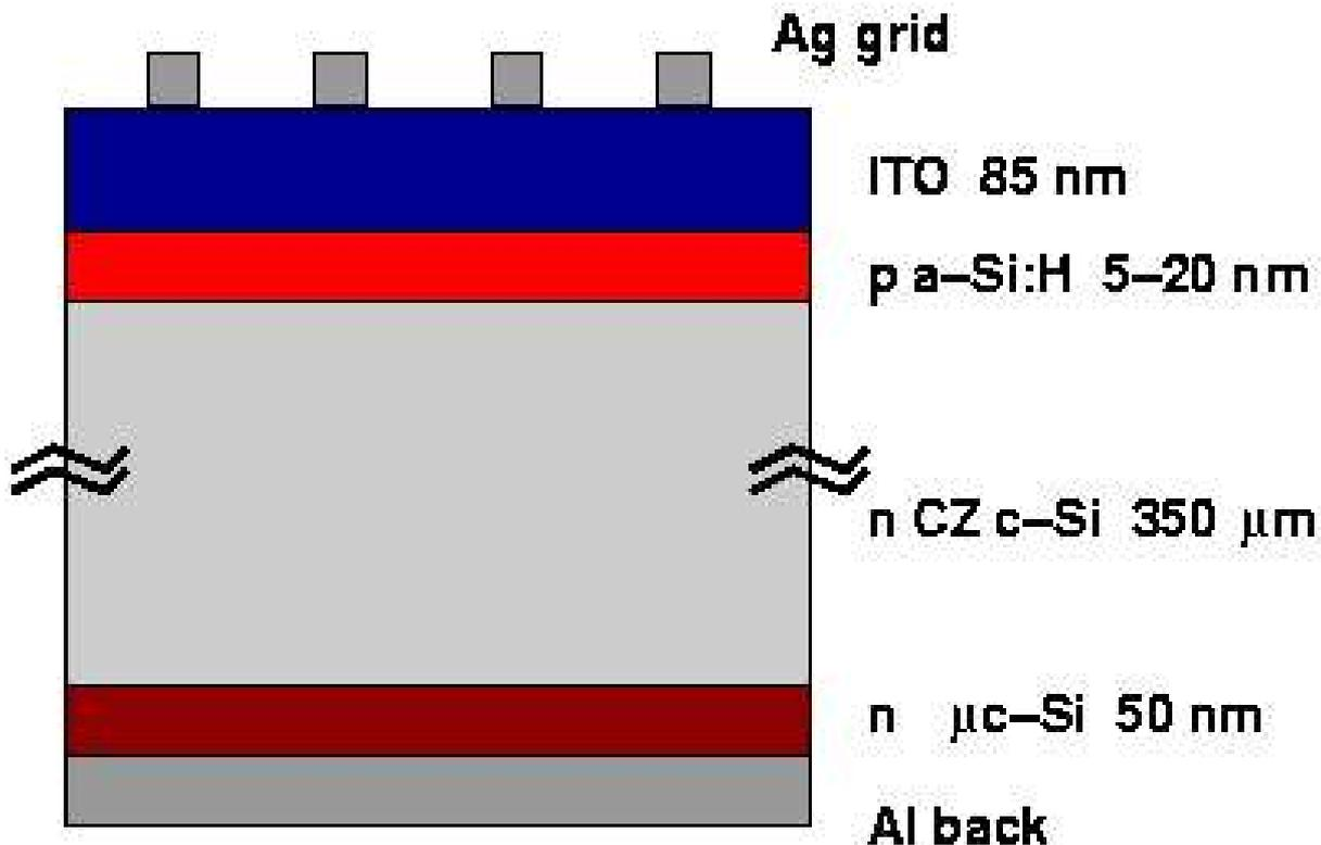
Simple low temperature process ( $< 250\text{ C}$ )
