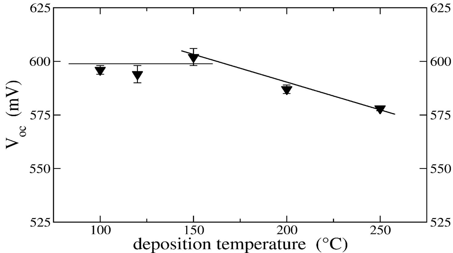
***Open circuit voltage vs. i epi-Si deposition temperature***
