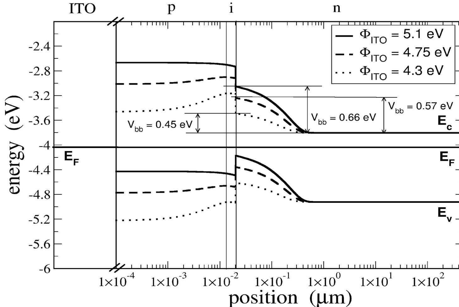
Computed heterojunction band diagram for different ITO work function at thermodynamic equilibrium. Software used: **AMPS**
