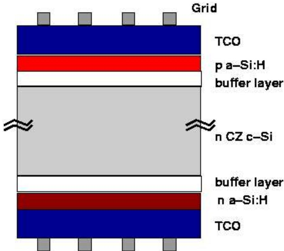
The passivation scheme can be applied also on the back side, a further improvement of performance has been demonstrated by Sanyo
