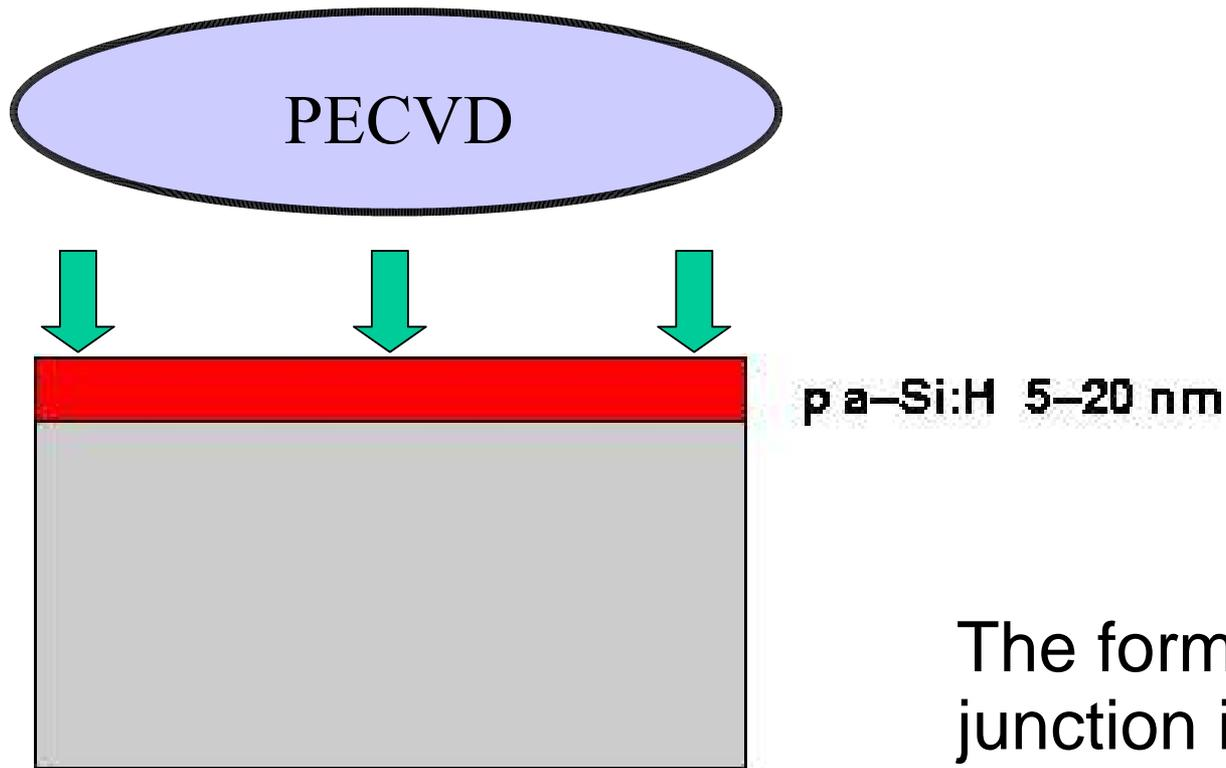
The formation of the p-n junction is obtained by PECVD deposition of a p type a-Si layer. The layer should be as thin as possible.
