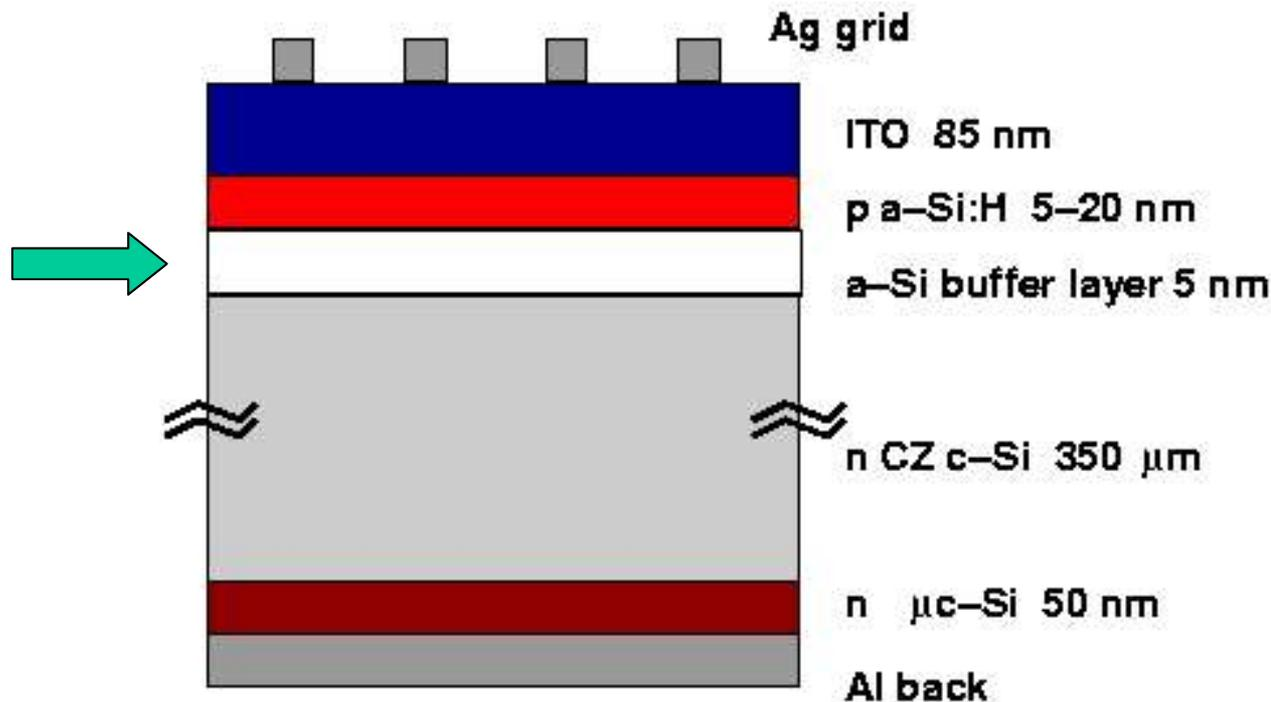
An intrinsic a-Si layer at the interface between p a-Si and n c-Si is used to reduce defect density.
