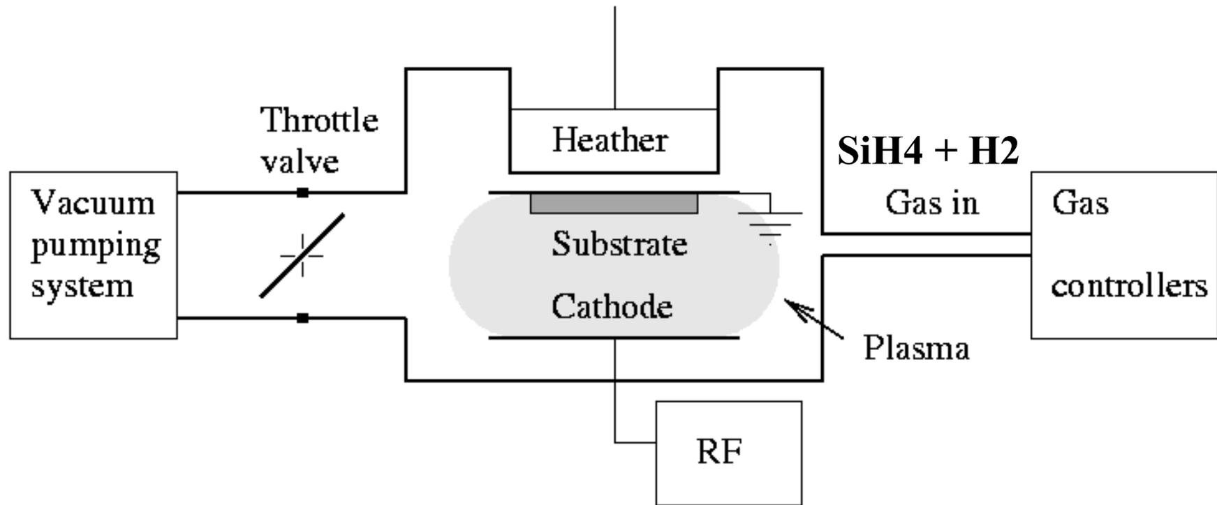
Low temperature process (plastic substrates, TFT display)
