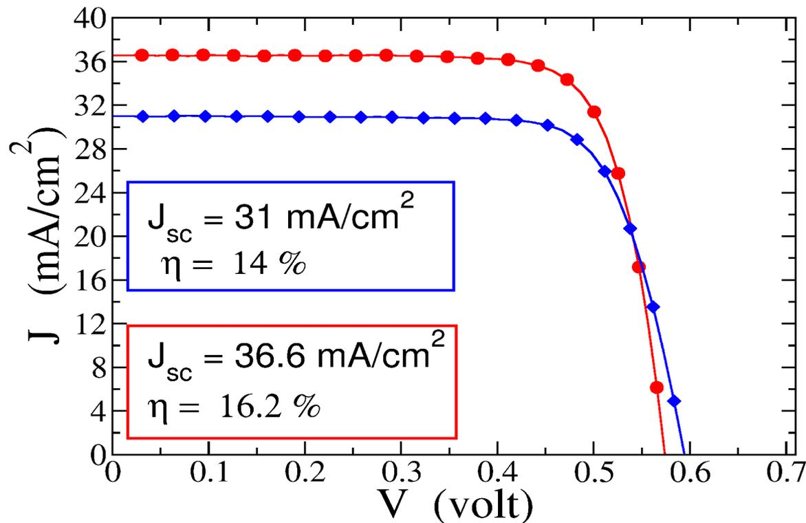
Using an *i epi-Si* buffer layer
