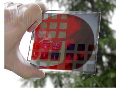
Thin film **amorphous** silicon solar cell:
