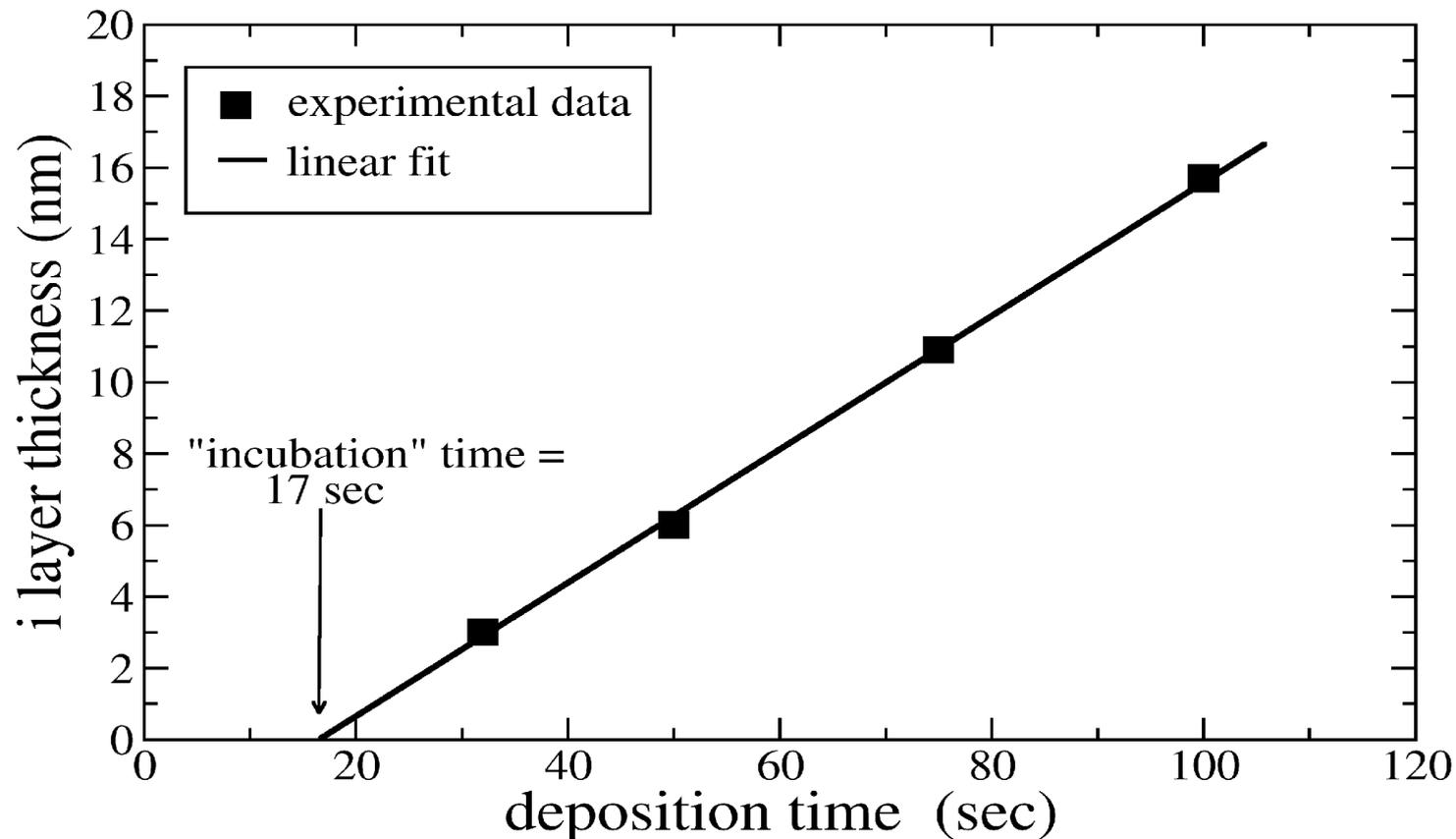
Amorphous silicon thickness for different deposition time. The substrate is crystalline silicon, the thickness was evaluated with spectroscopic techniques.
