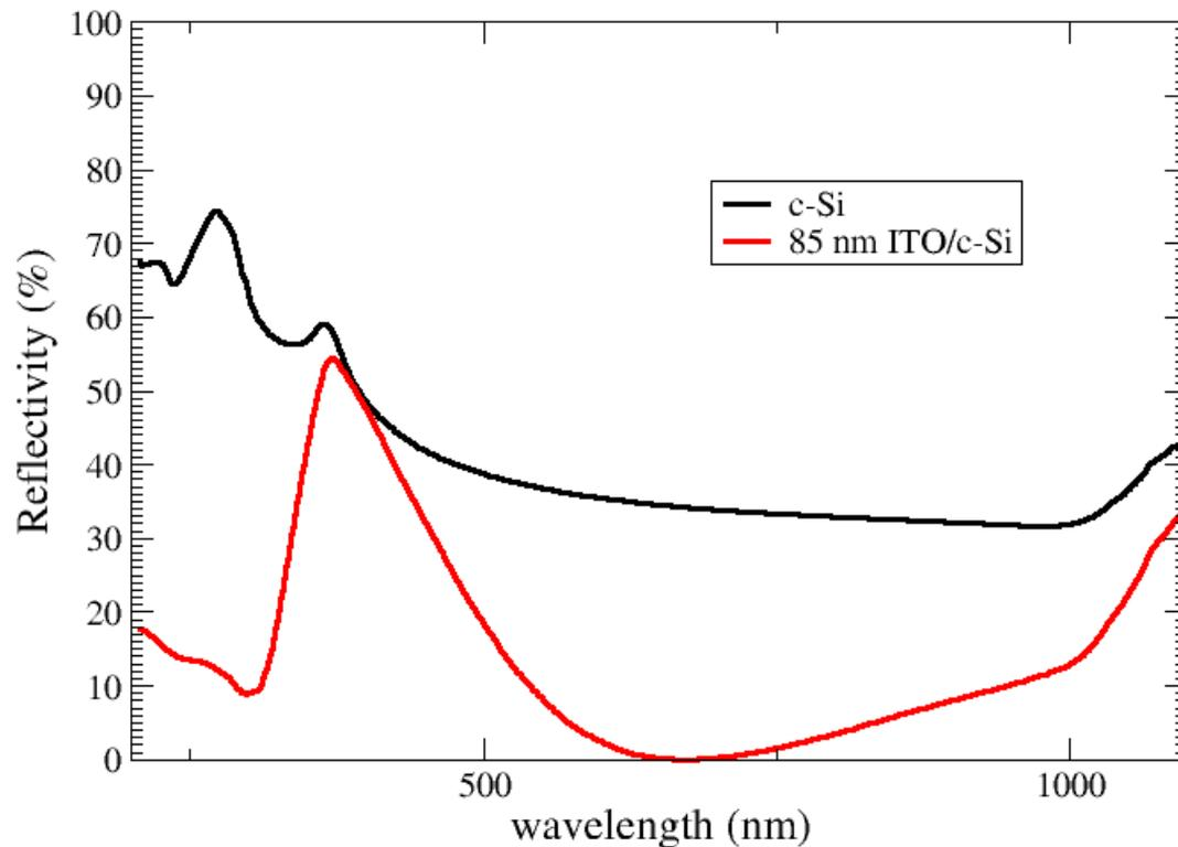
Indium tin oxide (ITO) has a good conductivity ( $2E-4$  ohm cm) that gives a sheet resistance of about 20 ohm square. Because the anti reflecting behavior the short circuit current increases of more than 30%.
