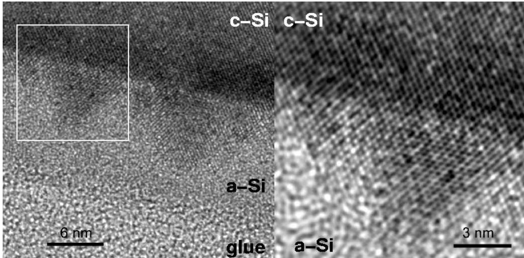
Cross section HR-TEM image of a-Si deposited on top of c-Si.
