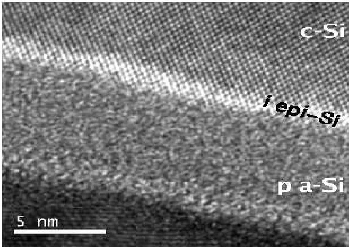
Epitaxial growth: condition close to chemical equilibrium i.e. etching rate close to deposition rate
