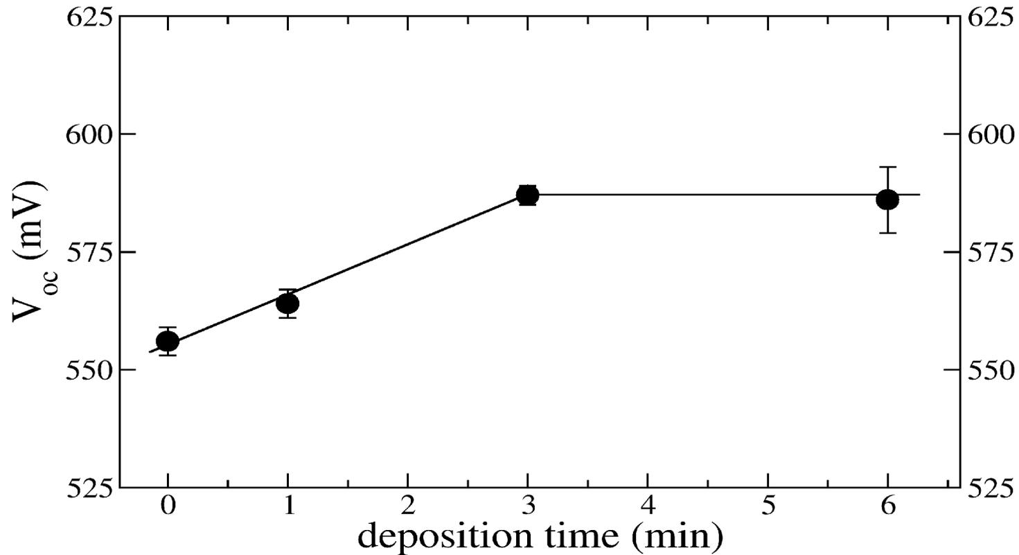
***Open circuit voltage vs. i epi-Si deposition time***
