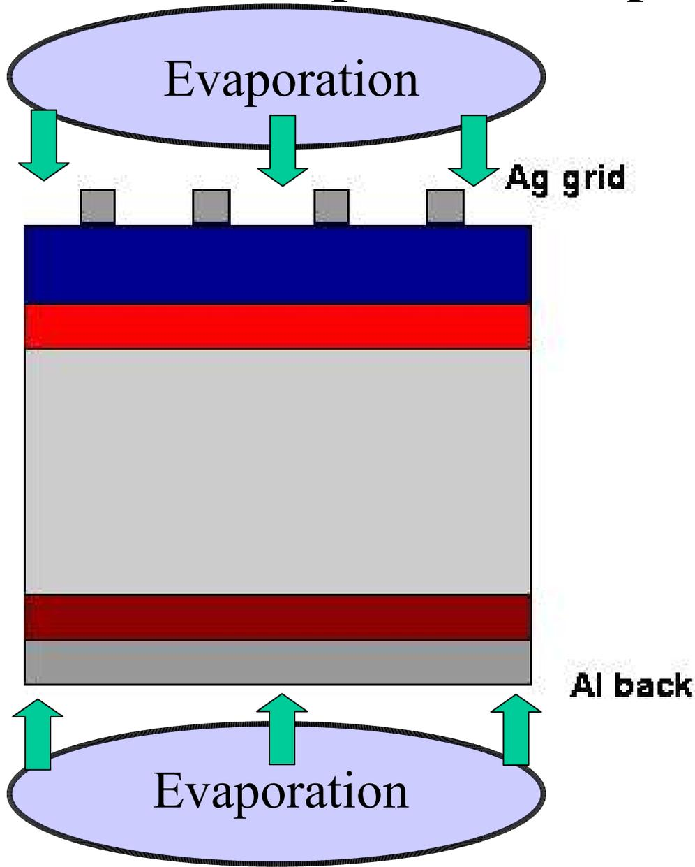
Electric contacts are obtained by thermal evaporation through metal mask. Low temperature screen printing technique can be also used.
