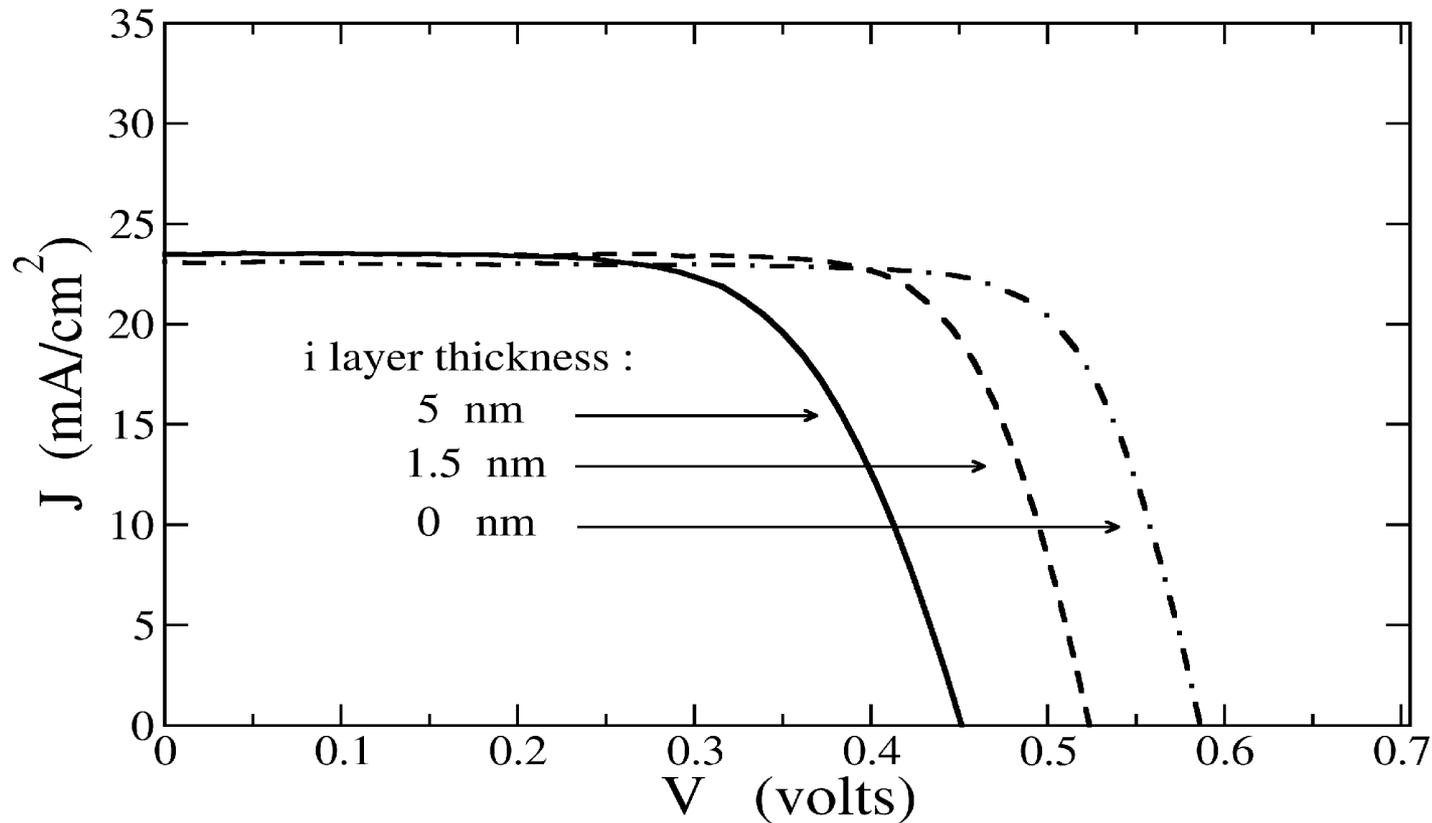
Experimental J-V curve for different thickness of “a-Si” buffer layer.
