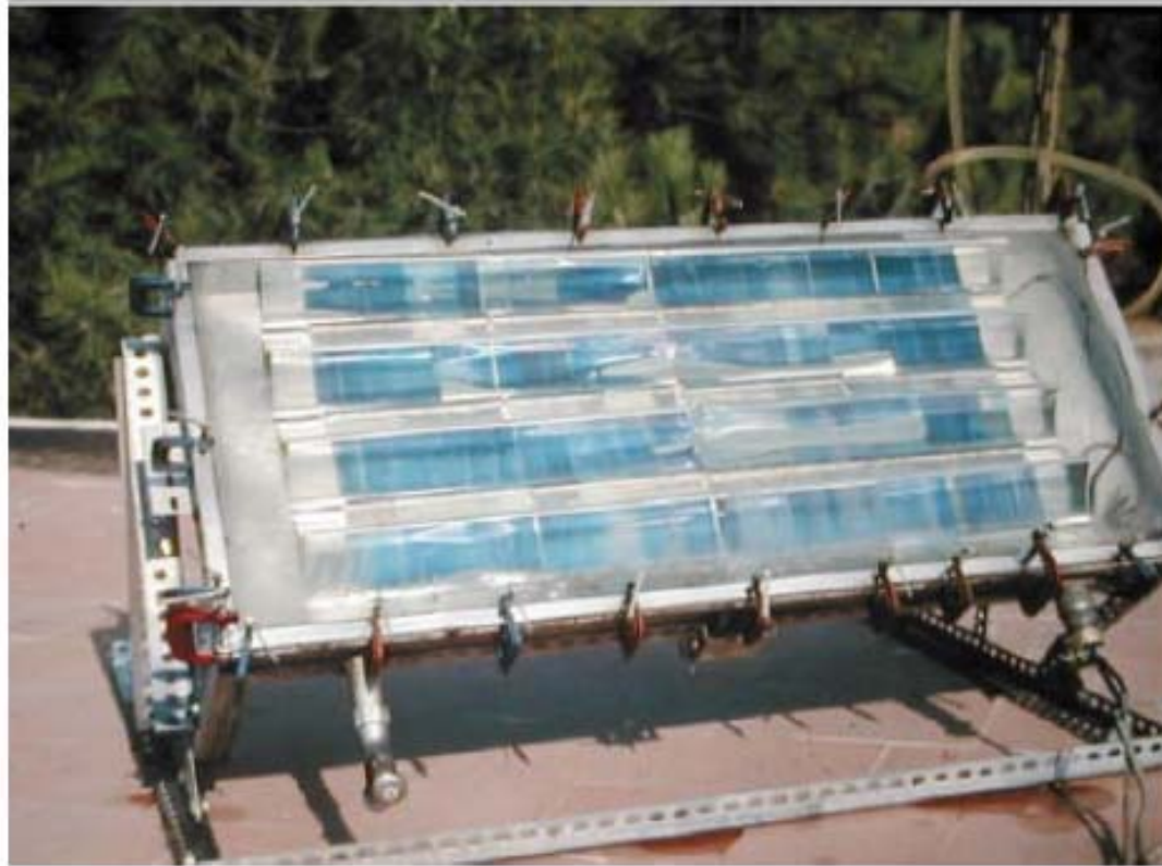
The prototype of the static concentrator (UPM-Universidad Politécnica de Madrid) with bifacial cells.
