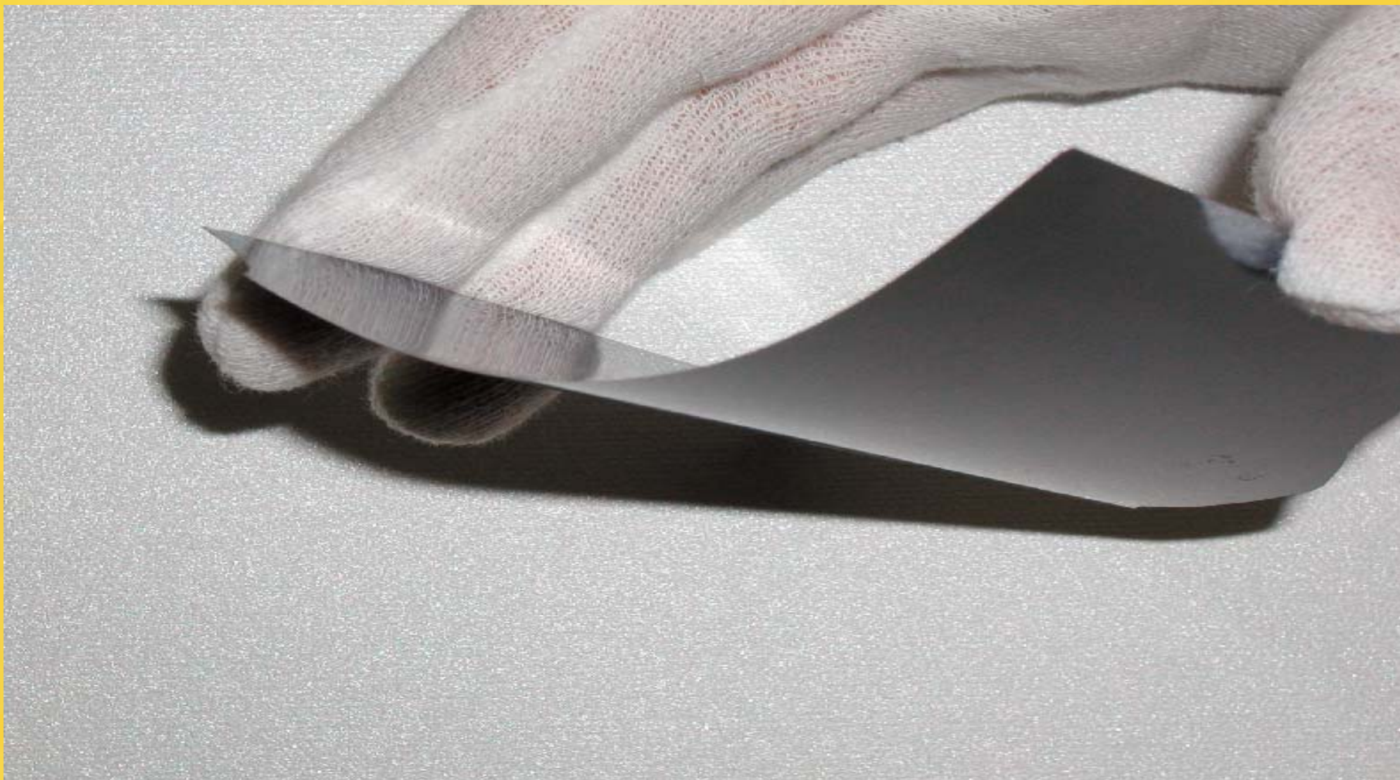
100 \mu\text{m} Thin and Flexible Wafer as Cut
