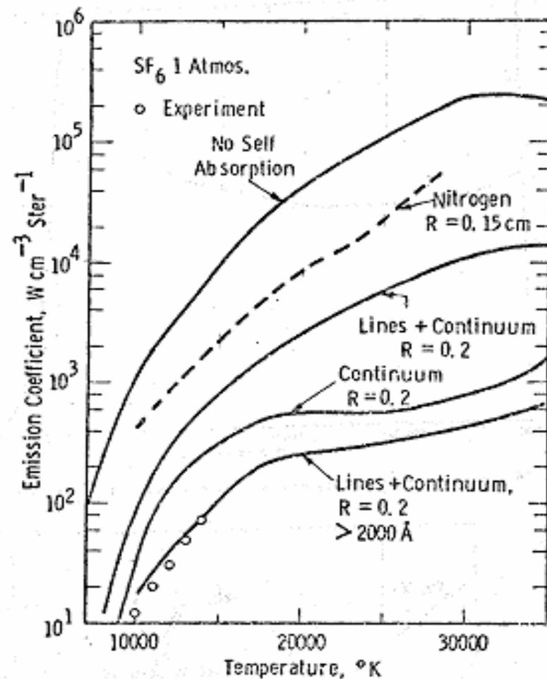
**Components of total radiation emission coefficient for  $SF_6$  at 1 atm.**
