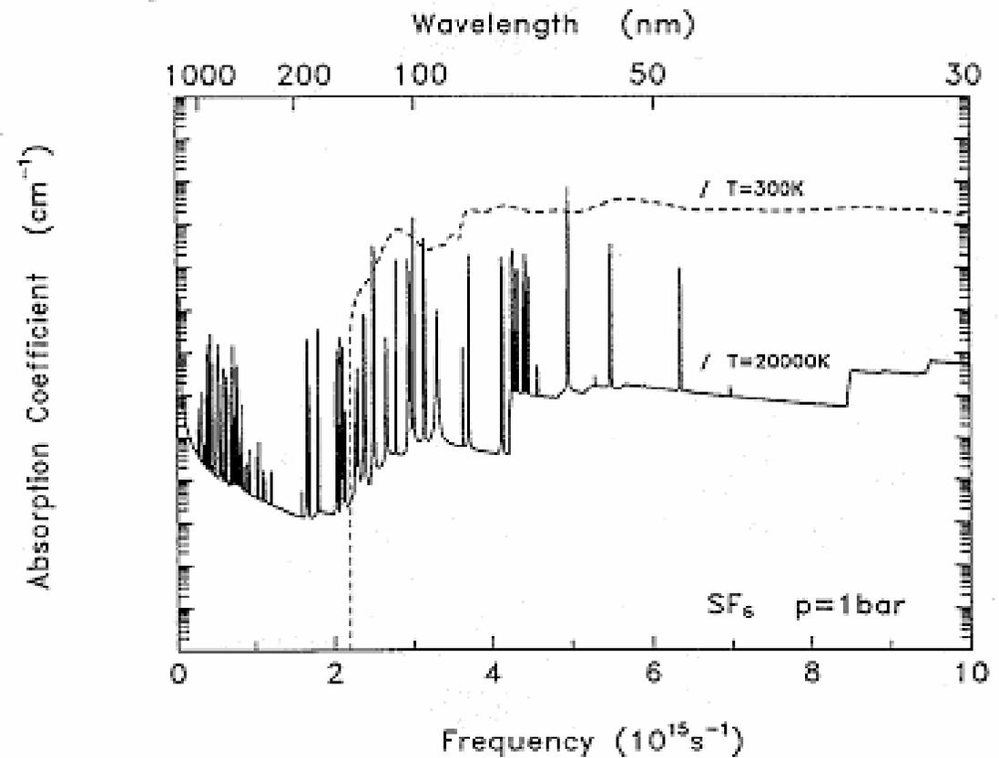
**Absorption coefficient of  $SF_6$  for temperatures of 300 K and 20 000 K**
