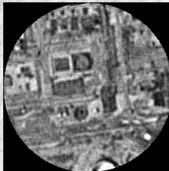
10°-rotated, 1.7X-magnified and P -th law spectrum compression enhanced ( P=0.5 ) image
