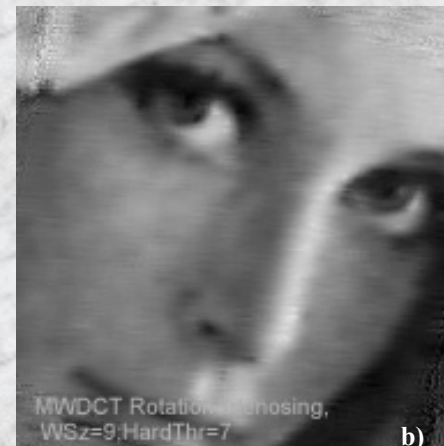
Noisy image (a) and a result of the rotation and denoising with sliding window DCT sinc-interpolation and denoising (b).
