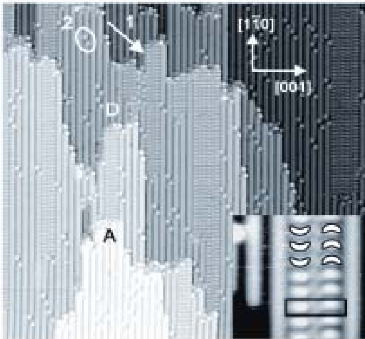
FIG. 1. Large-scale STM image showing coexisting molecular structures of D-cysteine on a Au(110)-(1 x 2) surface (425)
