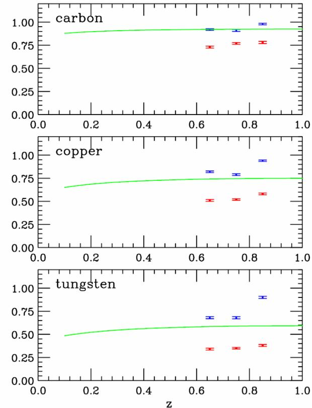
Figure 8: Attenuation of  $\pi^+$  (blue x, larger) and proton (red o, smaller) in carbon (top), copper (central) and tungsten (bottom) as a function of  $z$  for  $Q^2 = 2.81(\text{GeV}/c)^2$ ,  $\nu = 4 \text{ GeV}$  and  $P_T = 0-0.25 \text{ GeV}/c$ .
