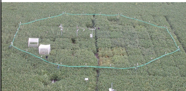
Free Air CO 2 Enrichment, FACE See Ainsworth and Long (2005) Photo courtesy of Steve Long, University of Illinois
