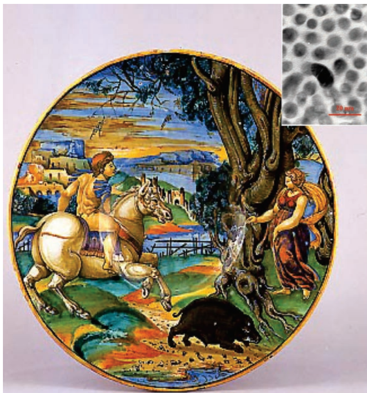
Fig. 23. – Lustre prepared by Mastro Giorgio in Gubbio (Italy, 1528) (Museo Civico della Ceramica di Gubbio, Italy). The inset is a TEM image of copper nanoclusters in the gold lustre.
