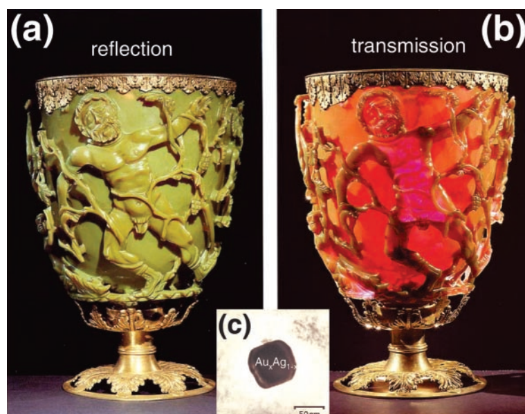
Fig. 22. – The Lykurgos Goblet (British Museum, Roman Glassmakers, 4th Century A.D.) illuminated under reflection (a) or transmission (b) condition. (c) TEM image of a Au-Ag alloy nanocluster inside the glass.
