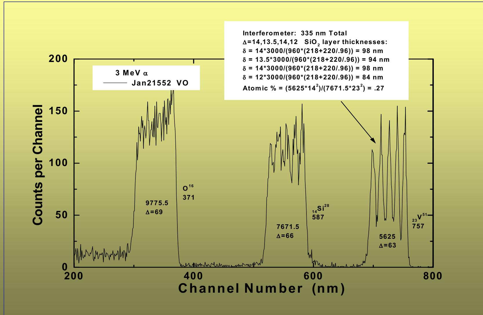
RBS spectrum of five Vanadium oxide layers in SiO<sub>2</sub> host
