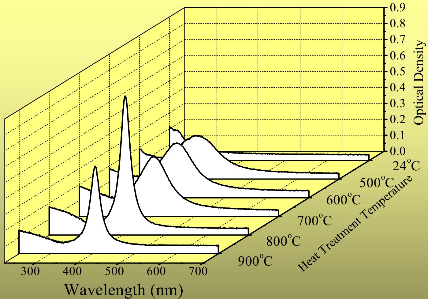
Optical Density vs. Wavelength after 1 hr heat treatments
