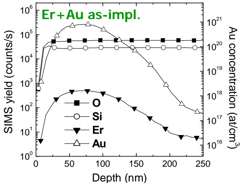
✓ Au and Er profiles overlapped after implant and also after annealing
