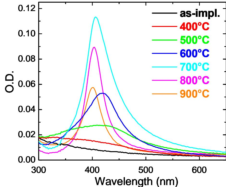
✓ Ag SPR band emerging as annealing T increases
