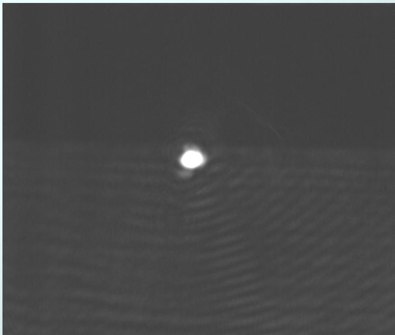
Near field image of a propagation mode at  $1.02 \mu\text{m}$  in a  $1.5 \mu\text{m}$  height  $\times$   $9 \mu\text{m}$  width ion-exchanged channel waveguide
