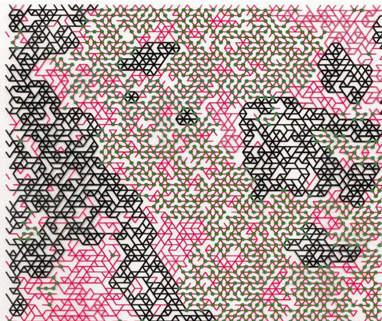
A typical section from a bond-diluted generic triangular lattice near the rigidity transition. Local distortions are not shown. A bond concentration of 0.66 yields large floppy and rigid regions. Green circles show pivot joints, and the black bonds are stressed.
