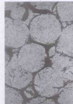
Sintered Fuel Pellets with black berry structure, low density and 'open' pores – suitable for LMFBRs
