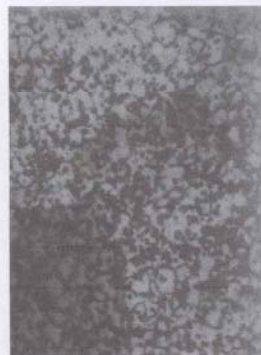
Sintered Fuel Pellets of High Density & Uniformly distributed 'closed' pores – suitable for PHWRs & LWRs
