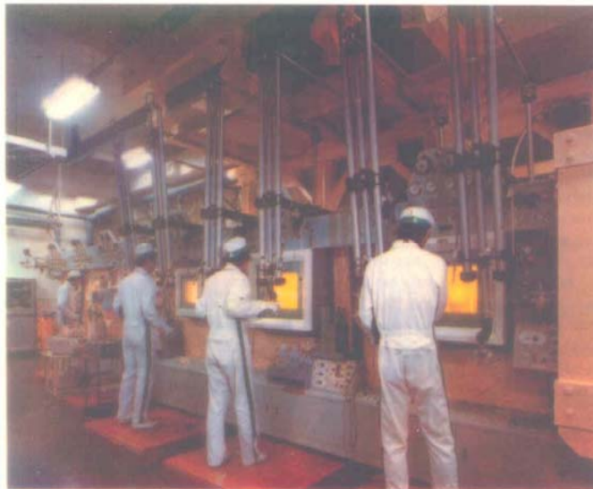
Remote Operations using manipulators for handling highly radioactive materials (mainly high gamma and high neutron dose) inside concrete hot cells
