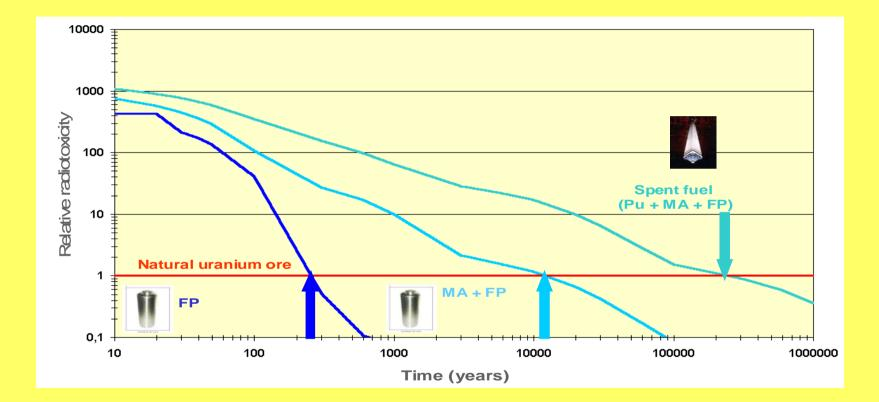
Instead of closing the fuel cycle only with Tu from spent fuels of thermal reactors with PUREX - a proliferation-sensitive technology — one might wait until fast reactors are in use and could transmute the Minor Actinides, MA, too.
