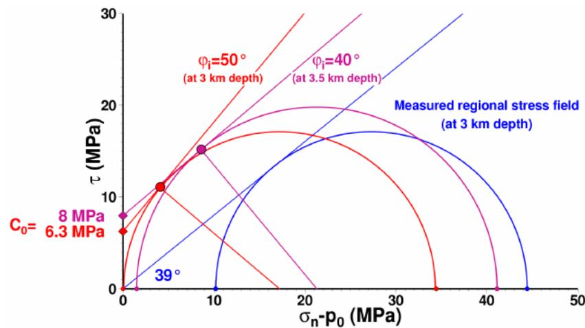
Evaluation of the rock mass permeability from the rate of growth of the microseismic cloud (Shapiro et al., 2000) yields pore pressure at time of failure inception
