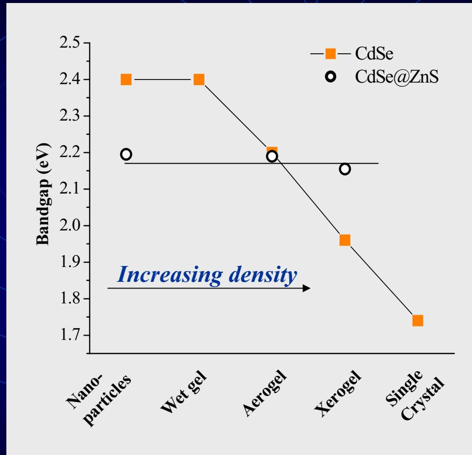
The presence of a ZnS barrier layer preserves the quantum confinement of the precursor nanoparticle, regardless of network density
