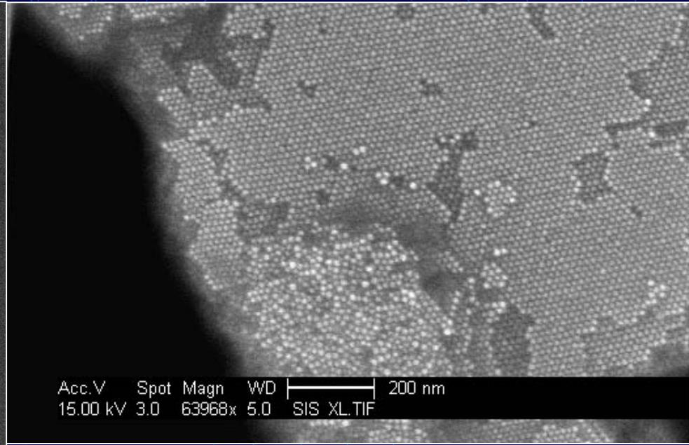
Colloidal crystal of ligand-capped gold nanoparticles held together by Van der Waals forces
