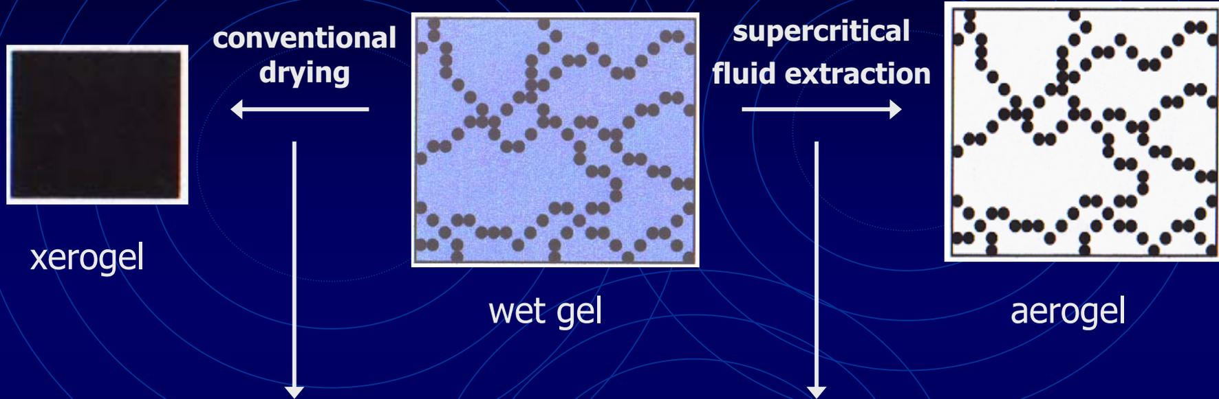
*Pore-collapse due to the action of capillary forces on the walls as the solvent evaporates leads to densification*
