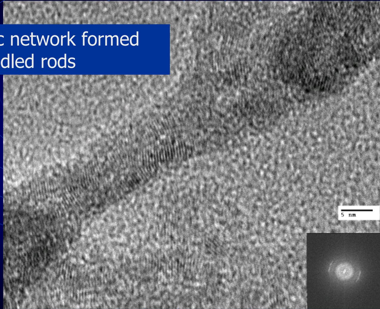
Lattice fringes =  $2.00 \text{ \AA}$  ,value for (103) plane of CdSe =  $1.98 \text{ \AA}$
