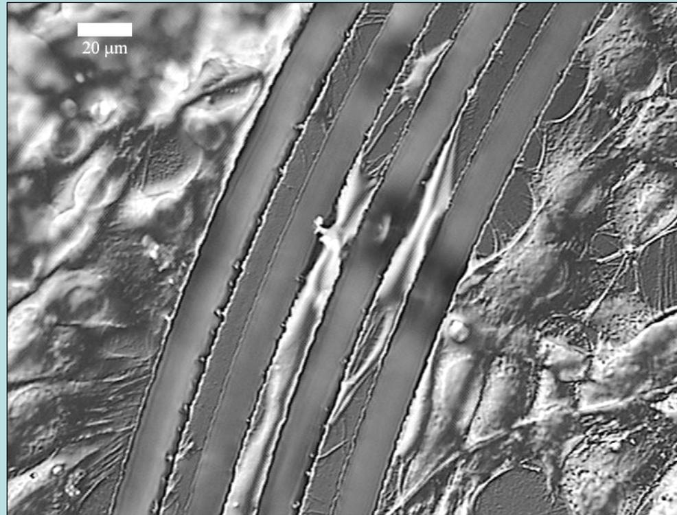
Cells align on ridge structures that are narrower than the natural cell width.... Tissue engineering applications
