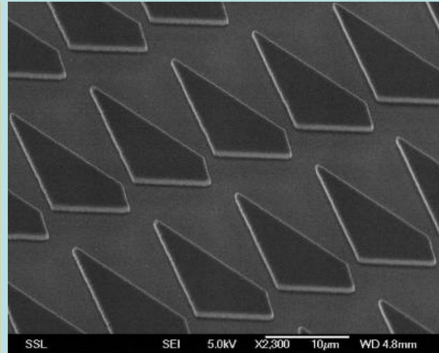
DNA – protein ratchet sorter: Using a combination of Brownian motion and Electrokinetic force, large molecules drift vertically through the obstacles, whereas the smaller molecules are ratcheted to the right.
