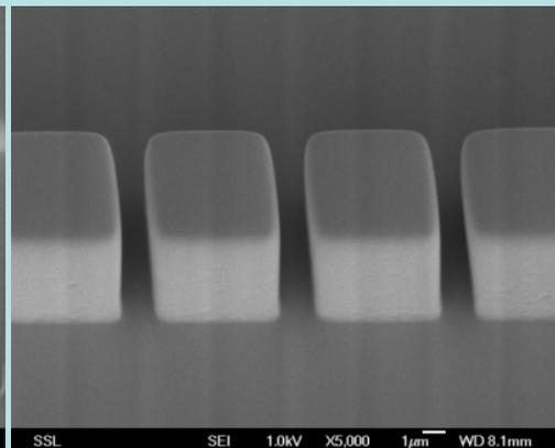
PDMS is poured into the mold, allowed to set, and released. The structure can be bonded onto glass eg to form a biochip cell sorter.....
