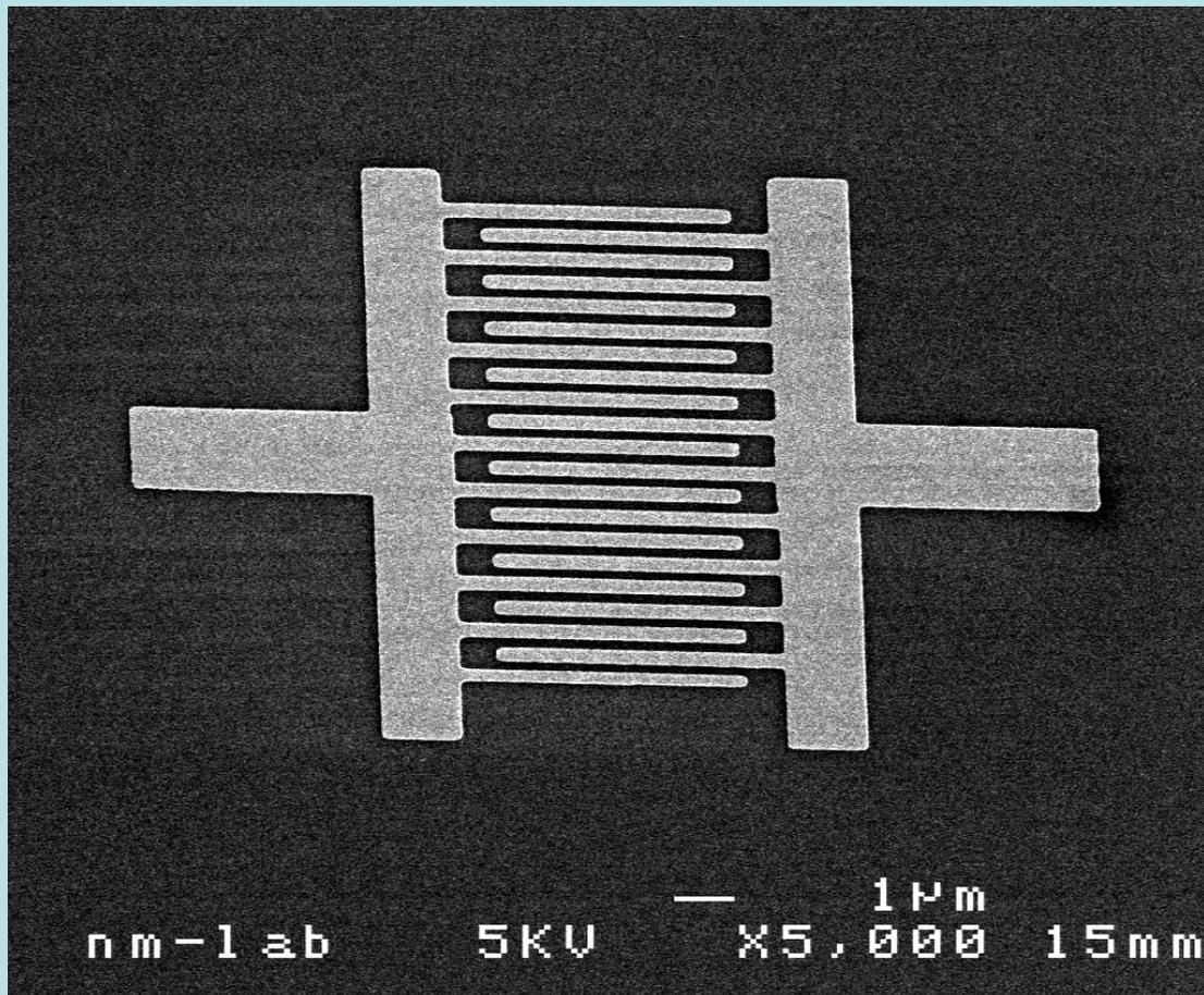
*Lithography of high spatial density biosensor structures with sub-100 spacing by MeV proton beam writing with minimal proximity effects.*
