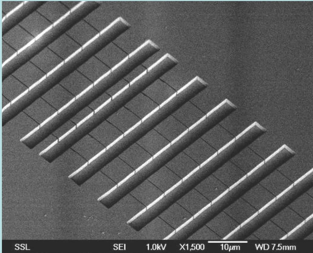
A series of reservoirs are connected by 100nm wide channels: When an electric field is applied along the channels, the DNA is stretched through the nanochannels at a rate which depends on the size and unfolding characteristics of the DNA.
