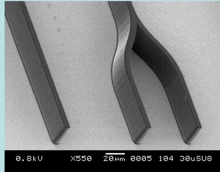
Test **waveguide structures** showing the side wall smoothness and orthogonality that can be achieved using p-beam writing. These structures were fabricated in a 30  $\mu\text{m}$  layer of SU-8 spin coated on a silicon wafer.
