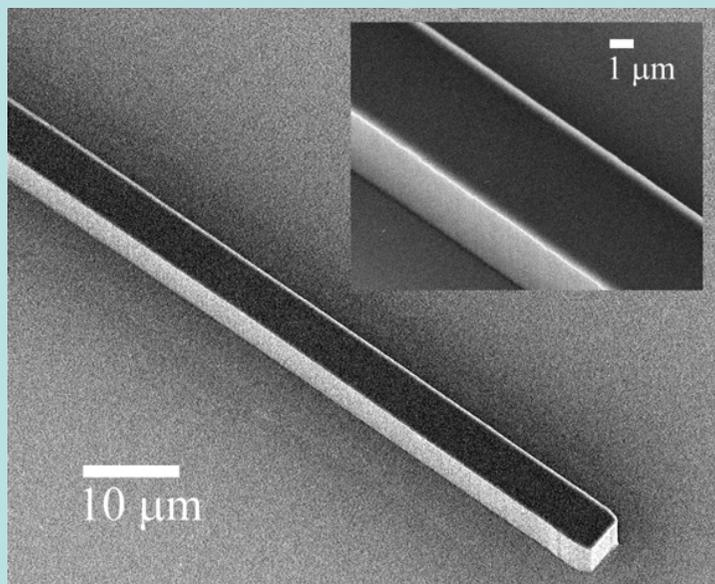
The waveguides fabricated using p-beam writing have smooth and vertical sidewalls, and exhibit low loss
