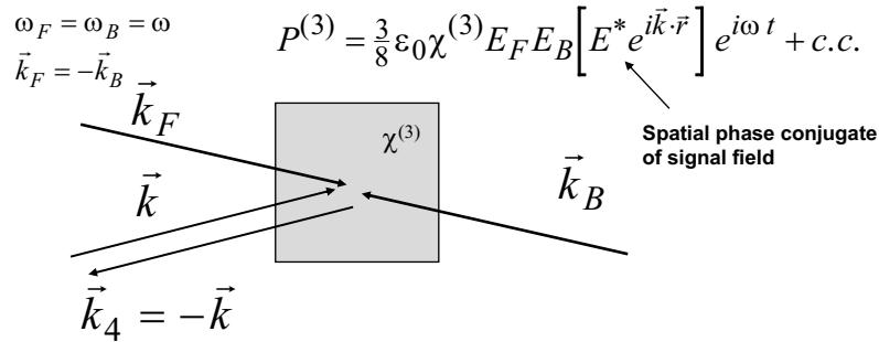
In fibers can be used to compensate dispersion and other time-phase distortions
