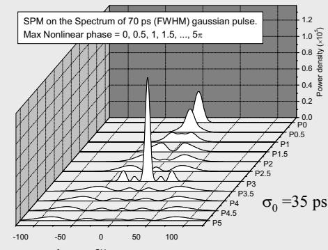
Spectra as a function of position ( $z$ ) for fixed input power, or as a function of power for fixed  $z$ .
