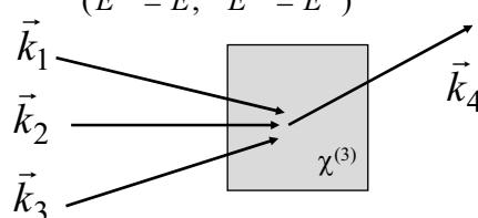
degenerated FWM:  $\omega_4 = \omega_1 = \omega_2 = \omega_3 = \omega$
