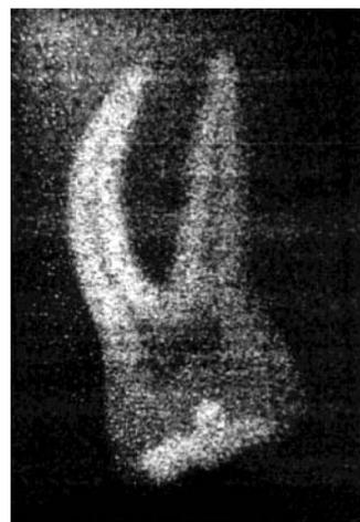
Figure 17. Latent X-ray image of a tooth in a Yb-Tm-doped vitroceraic, revealed by the blue emission under an IR irradiation at  $960 \text{ nm}$ .
