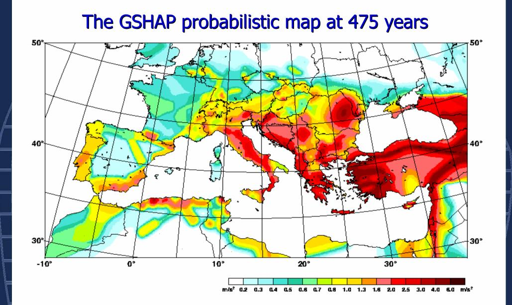
Horizontal Peak Ground Acceleration seismic hazard map representing stiff site conditions for an exceedance or occurrence rate of 10% within 50 years for the Mediterranean region.
