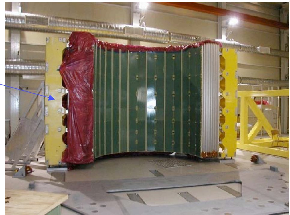
LAr EM barrel assembly in the vertical position
