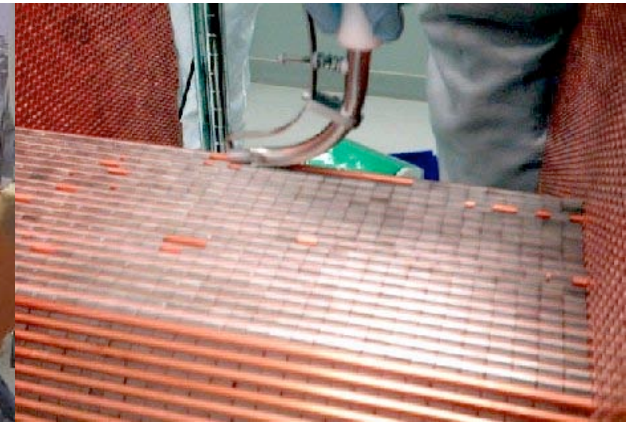
FCal2 and 3 assembly; insertion of tungsten slugs
