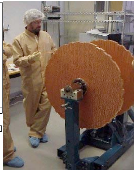
FCal2 and 3 assembly; insertion of tungsten slugs
